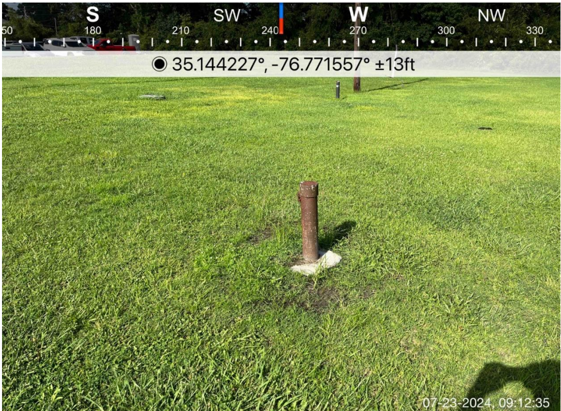
Photograph 4: Groundwater monitoring well (second well in the distance) in the northern portion of the site.
