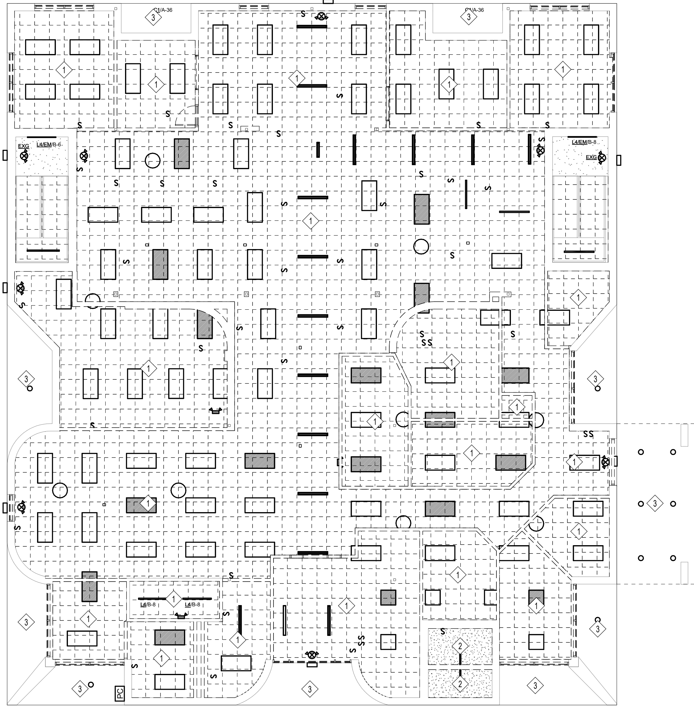
2 FIRST FLOOR DEMOLITION RCP 1/8" = 1'-0"
